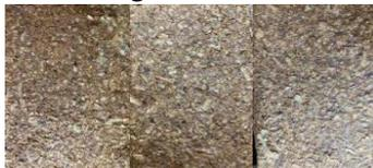
Gambar 4. *Natural oil – Biovarnish clear coat glossy – Biovarnish clear coat matte*
